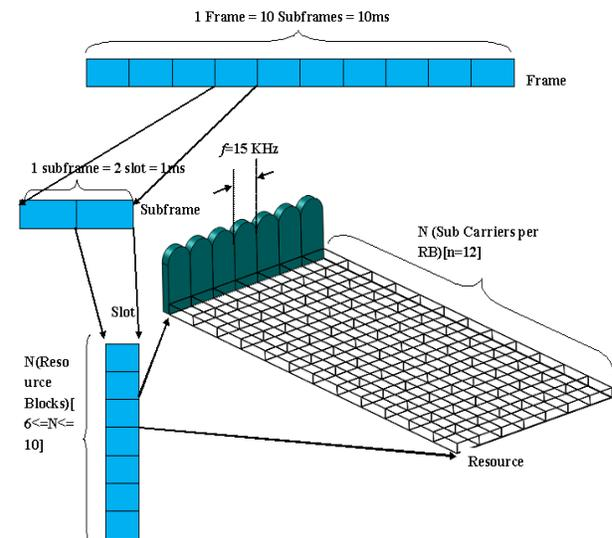
Figure 2. The structure and allocation of the eNodeB transmission resources symbols.
