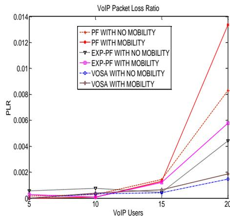
Figure 3. VoIP-Packet-Loss-Ratio Comparison
