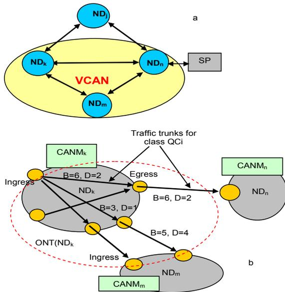
Figure 3. a. Inter-domain level overlay network topology (ONT); b. ONT of the domain NDk ( B= bandwidth, D= max delay- generic figures)
