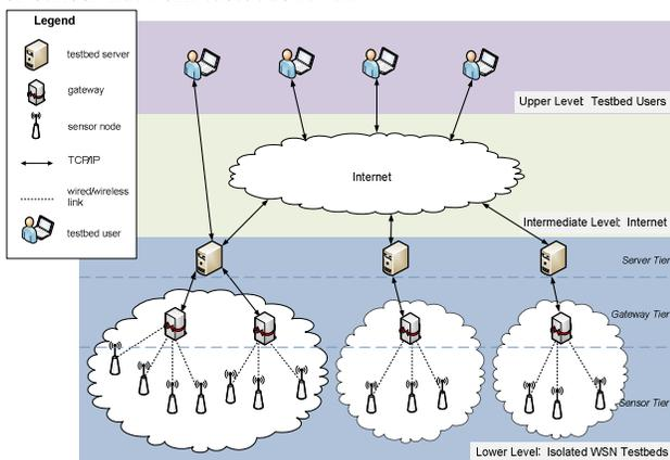
Figure 1: Reference architecture of federated WSN testbeds
