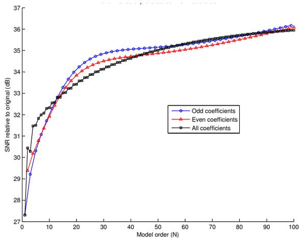
Figure 4. Distortion versus model order for odd-only, even-only, and odd/even model constructions with unit-valued coefficients.
