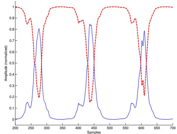
Figure 2. Estimated channel modulation envelope  $H_p$  (dashed line) and corresponding pre-distortion envelope  $\hat{H}_p^{-1}$  (solid line). Both signals are normalized to unit amplitude, and are shown prior to scaling for appropriate modulation depth.
