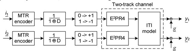
Figure 3. In-track MTR encoding over two-track channel.
