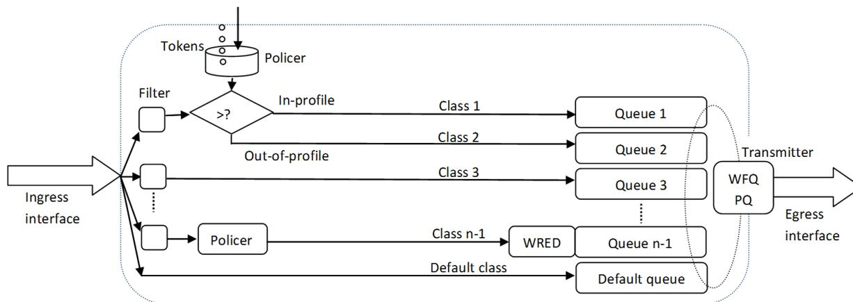
Figure 2. Illustration of QoS mechanisms in a router
