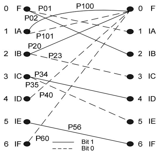
Fig. 4. Bit level trellis of RVLC decoder [10].
