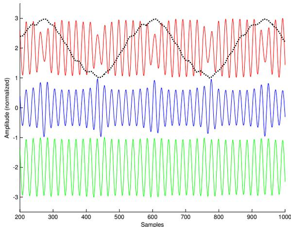
Figure 3. Top: distorted signal  $H_p(x)$  and power signal  $p(t)$  (dotted line); Middle: pre-distorted signal  $y$ ; Bottom: resulting signal  $\hat{x}$ , which approximates  $x$ . All signals are normalized to unit amplitude, and have been offset for clear display.
