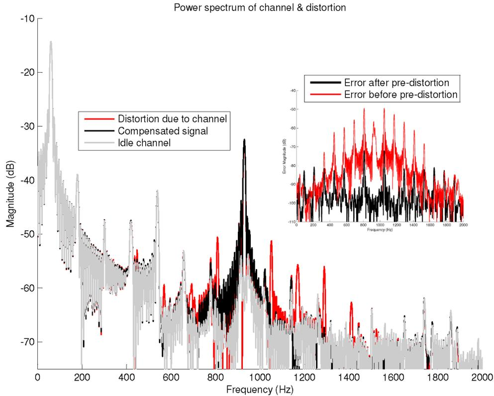
Figure 5. Power spectrum of channel before and after pre-distortion process via estimates of  $q$  and application of pre-distortion envelope  $\hat{H}_p^{-1}$ . The error signal spectra are shown in the inset. The spectrum of the compensated signal  $\hat{x}$  and the spectrum of the stimulus signal  $x$  are almost identical, and the channel-induced distortion is effectively suppressed.
