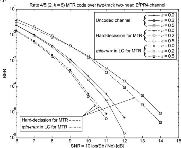
Figure 6. MTR decoding using *min-max* in LC.
