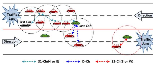
Figure 2. An Example of Wireless Communication Channels
