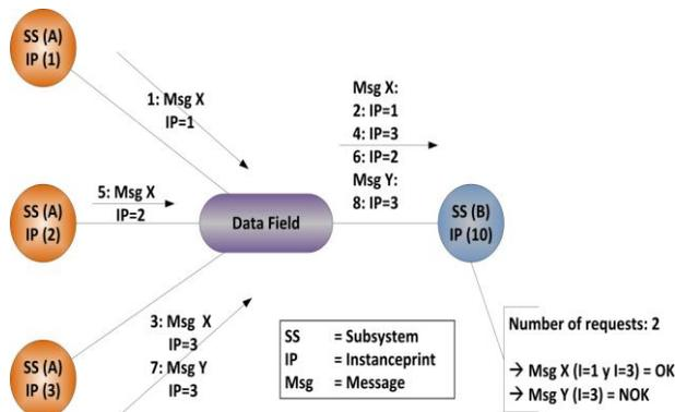
Figure 4. Receiving Multiple Requests from an Entity
