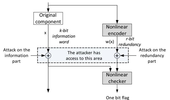
Fig. 2. Mathematical model of a circuit component protected by a systematic security-oriented code.
