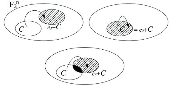
Fig. 3. The error  $e_1 \in E_a$  is always detected since  $\mathcal{C} \cap \{e_1 \oplus \mathcal{C}\} = \emptyset$ . The error  $e_2 \in K_d$  is never detected since  $\mathcal{C} = \{e_2 \oplus \mathcal{C}\}$ , and  $e_3$  is detected with probability  $Q(e_3) = |\mathcal{C} \cap \{e_3 \oplus \mathcal{C}\}|/|\mathcal{C}|$ .
