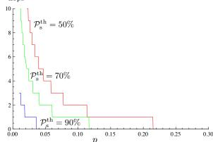
Fig. 7: Maximum sustainable number of hops with regular topology and for different values of the acceptable route probability of success.  $\theta = 10$ dB,  $\sigma = 4$ dB.
