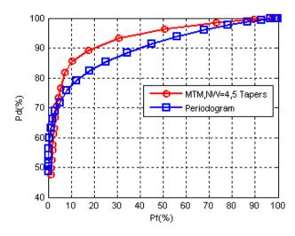
Fig. 7. Probability of detection versus probability of false alarm using MTM with *NW*=4 and *K*=5 tapers and periodogram using Rayleigh flat fading channel with SNR=- 5dB.
