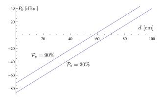
Fig. 2: Minimum transmission power as a function of the distance.
