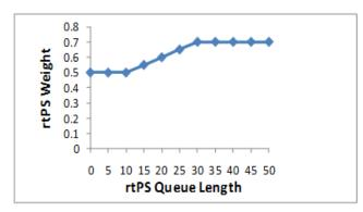
Figure 4. RED-based weights for rtPS service flow
