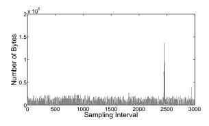
Figure 2. Number of bytes for a Streaming flow.
