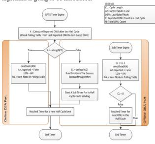
Figure 1. GATE Timer work flow in OLT
