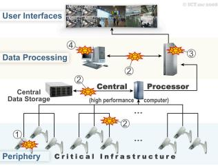
Figure 3: Attacks on a Single Site NIVSS
