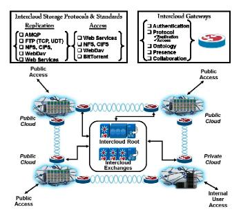
Figure 3. Intercloud enabled Federated Storage Architecture
