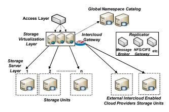
Figure 7. SSRP Enabled Cloud Storage Architecture
