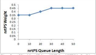
Figure 5. nrtPS weights of Enhanced RED-based WFPQ in Condition-1
