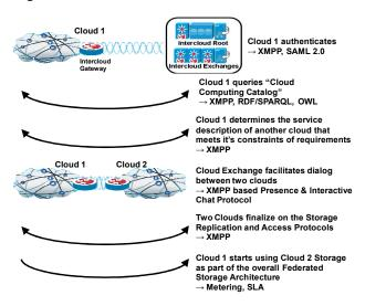
Figure 6. SSRP Unstructured Cloud Storage Sequence Diagram
