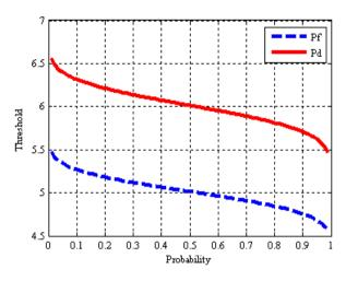
Fig. 4. Threshold versus probabilities of false alarm and detection using MTM with NW=4 and 5 tapers at AWGN with SNR=-7dB and L = 50 samples are used in the spectrum sensing.
