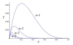
Fig. 6: Channel achievable transmission rate T in bits/s/Hz as a function of the hop distance (expressed in number of intermediary hop nodes n).  $\theta = 10$ dB,  $\sigma = 4$ dB, links SINR=10dB.
