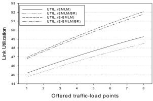
Figure 4. Link utilization for all models.
