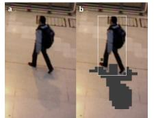
Figure 3: Shadow detection and cancellation. a, original image. b, detected shadow (gray blocks) and blob bounding box (white).
