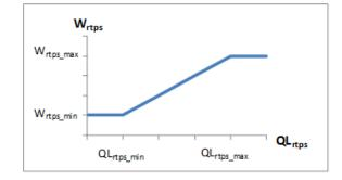
Figure 2. RED-based weights for rtPS service class
