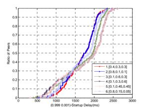
Figure 3. CDF of peers' (0.999,0.001)-Startup Delay with different [  $\omega_{C1}$   $\omega_{C3}$   $\omega_{C4}]$
