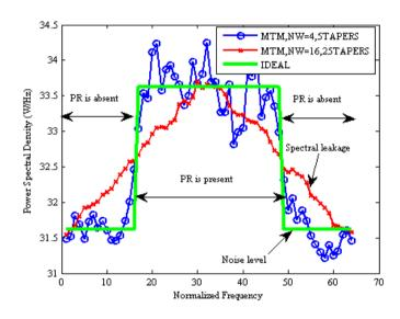
Fig. 2. Power spectral density (PSD) using MTM computed with NW=4, and 16 and different values of *K* at AWGN with SNR=-15dB.
