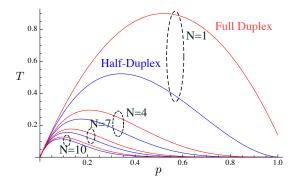
Fig. 4: Channel achievable transmission rate T in bits/s/Hz as a function of the number of nodes N connected to the hub.  $\theta = 10$ dB,  $\sigma = 4dB$ , links SINR=10dB.
