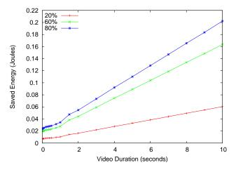
Figure 3. Saved energy as a function of video duration for different densities.  $\rho=1000$
