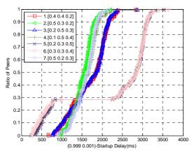
Figure 2. CDF of peers' (0.999,0.001)-Startup Delay with different [ $\omega_{B2}$  $\omega_{B4}$   $\omega_{B1}$ ]
