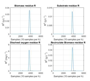
Figure 7. The residue, *R* for toxicity fault when N = 10
