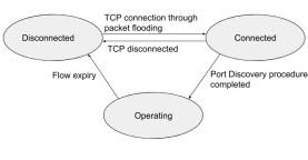
Fig. 2: State diagram of a switch/NE
