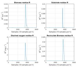
Figure 3. The residue, *R* for partial fault of the recirculation pump when N = 10
