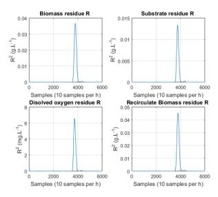
Figure 9. The residue, *R* for toxicity fault when N = 40
