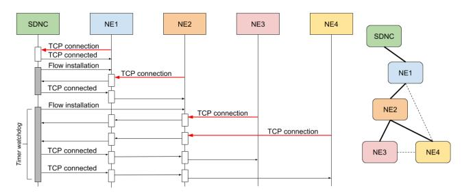
Fig. 5: Connection creation in a spanning tree of NEs using the proactive algorithm. See the text for detailed explanations.
