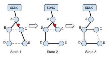
Fig. 6: A possible set of state transitions in the spanning tree as a result of superficial fault detection. See text for full details.
