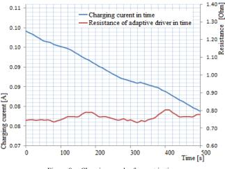
Figure 8. Charging graph of curent in time
