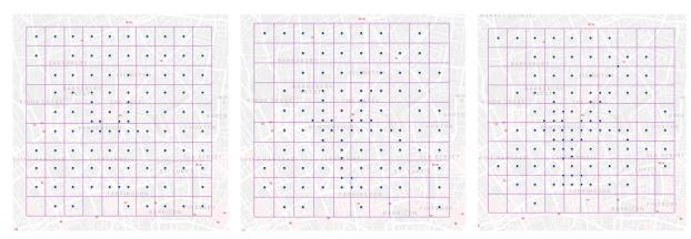
Figure 3. RSU Locations on Weighted Distribution Model for (a)  $\theta$ =10, (b)  $\theta$ =20, (c)  $\theta$ =30
