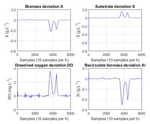
Figure 10. The outputs, *X*, *S*, *DO*, *X<sub>r</sub>* deviations caused by the toxicity fault  $(\mu_{max}/2 \text{ over } 3500 \text{ to } 3899 \text{ samples})$
