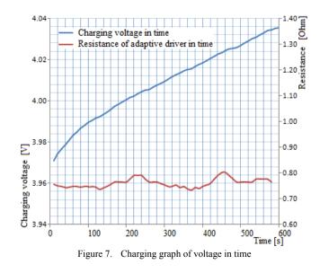
In Fig. 8 we are also highlighting the variation of adaptive resistance in time obtained in adaptive driver circuit. The variations of resistance of the adapter block are the answer due to the variations of internal resistance during the charging in time of the chemical element (battery).
