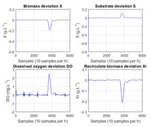
Figure 6. The outputs, *X*, *S*, *DO*,  $X_r$  deviations caused by the biomass sensor fault (X = 0 over 3500 to 3899 samples)
