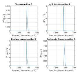
Figure 5. The residue, *R* for partial fault of the recirculation pump when N = 40
