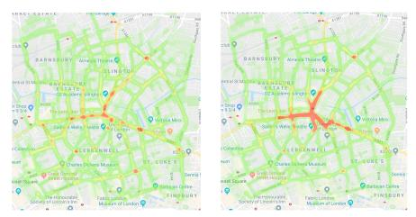
Figure 1. Heat maps of generated vehicle trajectories for the target area for number of vehicles (a) 500 and (b) 4000
