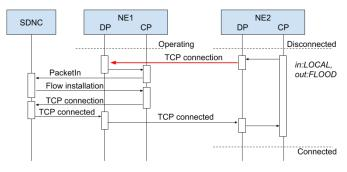
Fig. 4: Protocol elements for lower-tier NEs connecting to the SDN via a higher-tier NE
