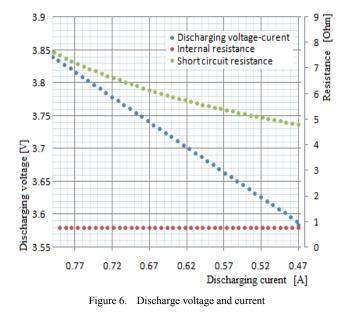
Numerical differentiation of the experimental data has led to the determination of the value of the internal resistance  $R_0 \simeq 0.76\Omega$
