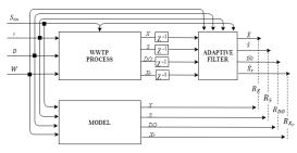
Figure 1. The fault detection scheme
