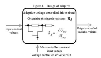
The electric circuit contains an active element whose transconductance and dynamic resistance introduced in the circuit can be controlled by a command voltage applied to the command pin of the active element in order to achieve dynamic charging. The input of the circuit is connected to the constant voltage generator and the output provides control of the output resistance, by controlling the output voltage and current.
