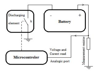
Figure 2. Discharging and testing circuit
