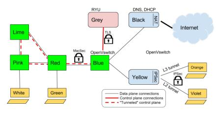
Fig. 1: Current SDN laboratory configuration
