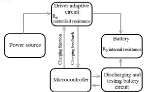
Figure 1. Block schematic of the proposed solution
