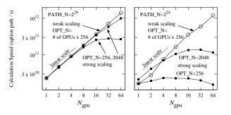
Figure 5. Performance of MonteCarloMultiGPU, an implementation of the Monte Carlo approach to option pricing, included in the CUDA SDK. Calculation speeds are plotted against the number of GPU devices,  $N_{\rm gpu}$ . The number of options calculated for is denoted by OPT\_N. The number of integration paths is denoted by PATH\_N. Weak scaling graphs show good scalability for both cases, but for strong scaling with smaller calculation cost shown in right panel is worse.
