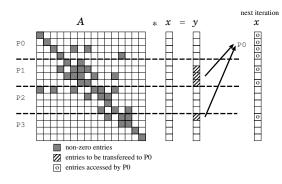
Figure 2. A Sketch of Communications for Transferring Minimum Block of Data Necessary for the Next SpMxV.
