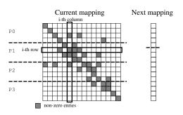
Figure 3. A Diagram of Determining the Target Process of Communications for an Entry.
