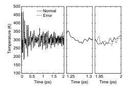
Figure 7. Temperature of a system from a molecular dynamics simulation is plotted against time (pico second). Middle and right panels are a closeup of the left one. Solid curves (Normal) show the correct result, while dashed curves (Error) show the result including errors.
