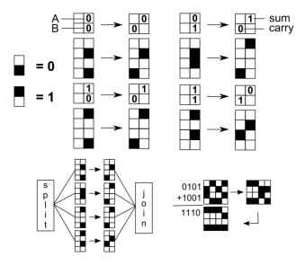
Figure 3. Realization of a ripple carry adder with SSL. For reasons of improved robustness a dual rail coding is used for 0 and 1.
