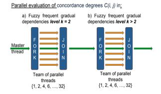
Figure 5. Parallel evaluation of fuzzy concordance degrees in: a) Gradual dependency of level k = 2, b) Gradual dependency of level k > 2.
