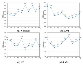
Figure 2. Comparison of DBI values for various v in the OT dataset. The salient features were selected by our method and were used to perform clustering using (a) *K*-means, (b) SOM, (c) HC and (d) PAM algorithms. The parameter  $v = \{10, 20, ..., 100\}$  was set to observe the corresponding performance.
