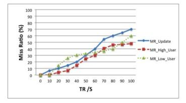
Figure 3. Transaction Miss Ratio (MR) when using EDF, with one single queue  $% \left( {{\left[ {{K_{\rm{B}}} \right]} \right]_{\rm{T}}}} \right)$
