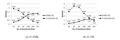
Figure 7. Comparison with PCR (Parallel Cyclic Reduction)
