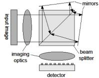
Figure 2. Implementation of SSL with optical hardware.
