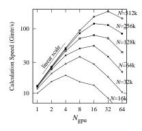
Figure 6. Performance of gravitational many-body simulations. The number of pairwise interactions between two particles calculated per second is plotted against the number of CUDA devices,  $N_{\rm gpu}$ , for various number of particles in the system, N.
