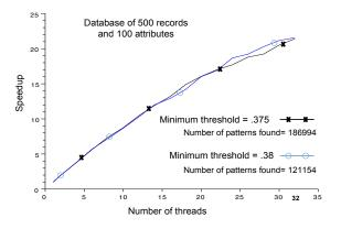
Figure 7. Speedup with a database of 500x100 and minSupp=.375 and .38, using uncompressed binary matrices of concordance degrees.
