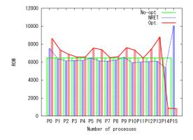
Figure 4. Fluctuation of Number of Rows Attached on each Process for matrix matrix\_9.
