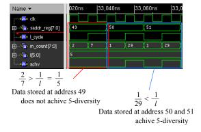
Figure 3. Observed waveforms
