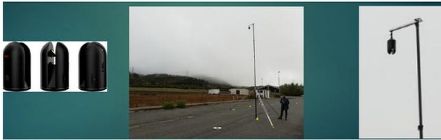
Figure 3. BLK36 scanner mounted on pole in tripod
