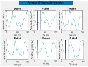
Figure 5: VEP changes during sample collection using GUIDE interface for a 6-month-old infant with vertical lines to mark the stimulus presentation (black) and the ideal P100 latency (blue). Each graph corresponds to adding 20 epochs to the signal processing from left to right.
