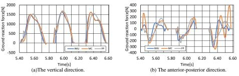
Figure 3. The GRFs estimated using 5 IMUs or MC. Here the GRF during the aerial period are corrected.
