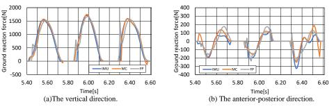
Figure 2. The GRFs estimated using 15 IMUs or MC. Here the GRF during the aerial period are corrected.
