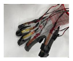
Figure 2. A homemade bending and pressure sensing glove.
