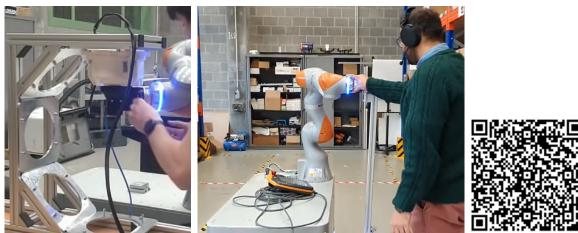
Figure 8. (Left) AMR in a 3<sup>rd</sup> hand configuration, (Middle) AMR in Joystick configuration, (Right) QR code of a video with the 2 realizations
