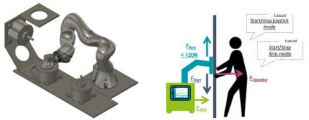
Figure 3. (Left) AMR configuration as a 3<sup>rd</sup> hand to support Operators, (Right) AMR configuration as a 'joystick' for part's transportation and handling with extended reach
