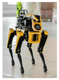
Figure 1. SPOT robot as an example of an AMR.
