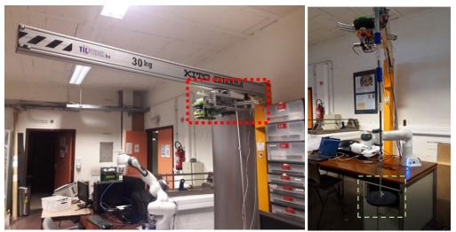
Figure 5. Jib crane with a gravity compensator (left – red dash line) coupled to a Franka Emika Panda Cobot (right). The payload of the cobot is initially 3kg (the gripper weighting already 0,8kg) and the manipulated load (black cylinder – green dash line) weighs 5kg
