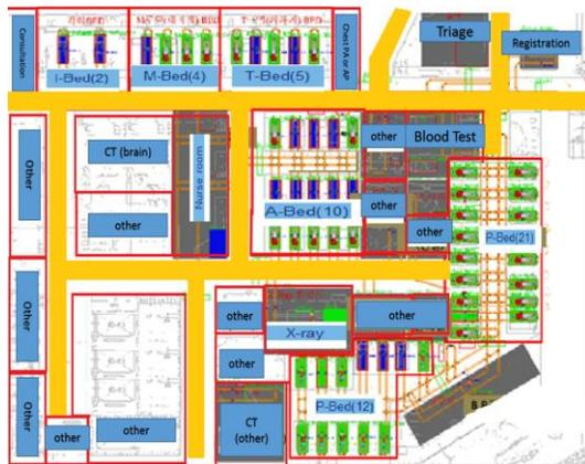
Figure 6. Optimum layout of ED.
