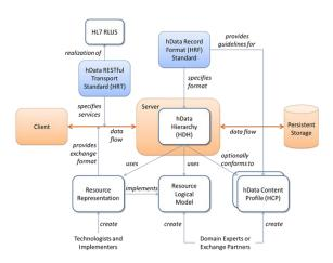
Figure 6. Relationship between the different components of hData [13]
