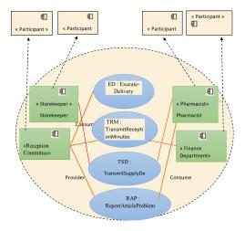
Figure 4. SoaML architecture diagram
