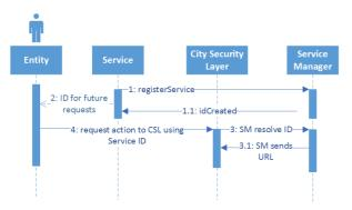
Figure 4. Sequence diagram with the workflow between CSL and Service Manager
