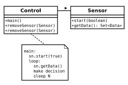
Figure 1. An example—class diagram.
