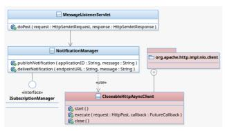
Figure 5. Message Listener Component Class Diagram
