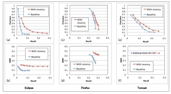
Figure 1. Performance of recommendations by considering of recency and baseline with varying minconf. The upper graphs show a relation between  $Precision_M$  and  $Recall_M$ . The lower graphs show a relation between MRR and  $Recall_M$ .
