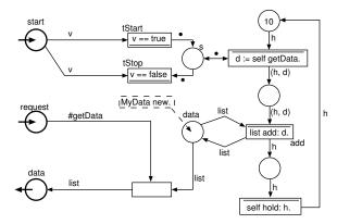
Figure 4. OOPN model of the component Sensor
