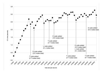
Figure 10. Near-real-time, full ETL system scale-out
