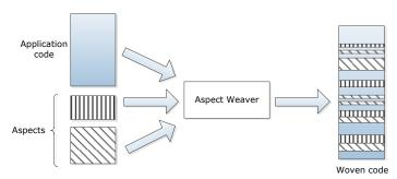
Figure 1. Illustration of how aspects are maintained outside the target application code, and then are intermixed with it.
