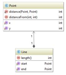
Figure 1. Reference UML class model (Diagram 1).
