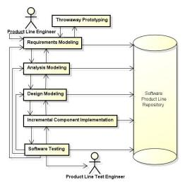
Figure 1. Process for applying the PLUS approach to SPL Engineering
