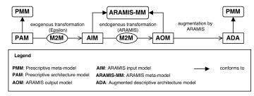
Figure 2. The model transformation chain in ARAMIS.
