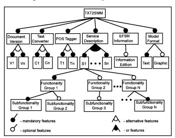
Figure 4. Feature diagram for the txt2smm system.
