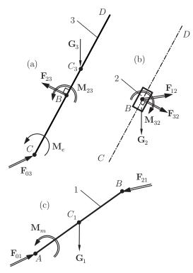
Figure 3. Free body diagrams for each link.
