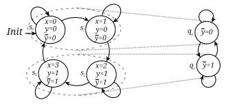
Figure 2. Constructing the quotient STS using the refinement mapping  $\frac{1}{2} \stackrel{\triangle}{=} u$
