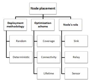
Figure 1. Sensor node placement methodologies
