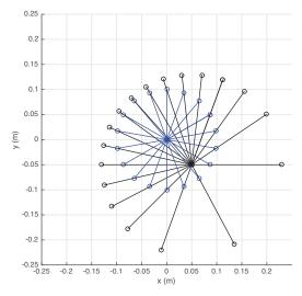
Figure 2. MATLAB representation of the R-RTR chain for a complete rotation of the driver link.
