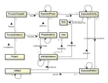
Figure 3. Process Model derived from SPEM
