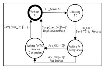
Figure 7. EFSM manually generated. Adapted from [33]
