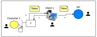
Figure 1. Authentication-flow with SAML.
