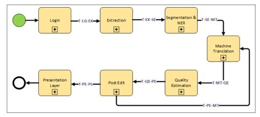
Figure 1. Workflow design of content process.
