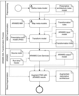
Figure 3. The ARAMIS ADL transformation process
