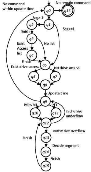
Figure 8. Cache program state transition diagram
