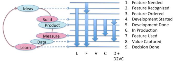
Figure 1. The value-driven metrics framework for driving software engineering cycle-time reduction (on the right), the Lean Startup cycle (on the left) and example cycles, for which cycle time can be used as the metrics driving cycle-time reduction (in the middle).
