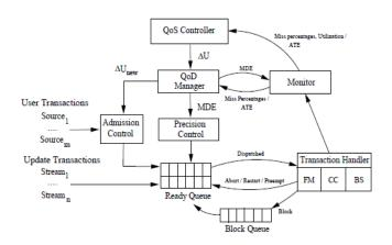
Figure 1. Basic Feedback Control Scheduling Architecture in RTDMS.
