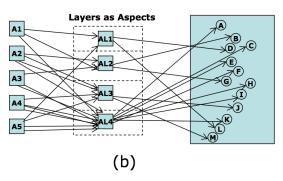
Figure 2. Aspects defining pointcuts (circles) on the reengineered system that are logically grouped in intermediary abstractions (layers as apects) that can be used to "visualize" the system's layers.
