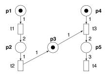
Figure 2. Example of a Petri net model
