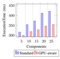
Figure 9. Execution times of two types of systems when processing an image with 1152\*864 pixels
