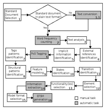
Figure 2. Process Diagram for State Machine Generation.
