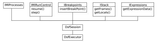
Figure 3. Main interfaces of CDT's debugger service framework.
