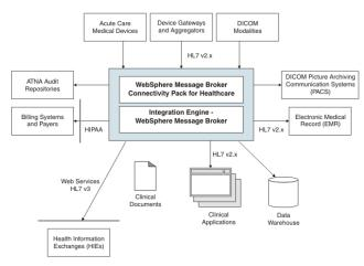
Figure 8. Architecture of a health system using WMB [12]
