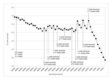
Figure 11. Near-real-time, full ETL system scale-in
