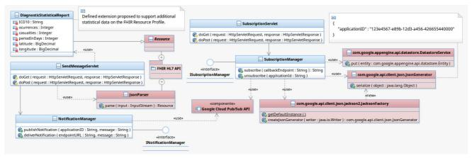
Figure 3. Subscription & Notification Scenario Class Diagram.
