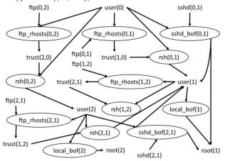
Figure 4. Example Condition/Exploit-Oriented Attack Graph
