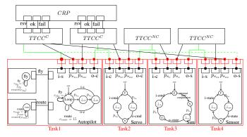
Figure 10. Final Flightsim model
