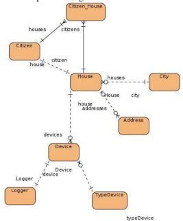
Figure 4. Design of the PlugTV database.
