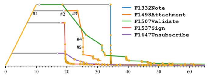
Figure 3. Depiction of the cycle-times of the five features. Development working days share the rising line starting from (event 5) and end in event 6 (start of the gray horizontal line), deployment (7, white dots in the right end of the gray part of the horizontal lines) and usage (yellow dots). To enable comparison, all the features are synced to have event 5 (start of development) at day 0.
