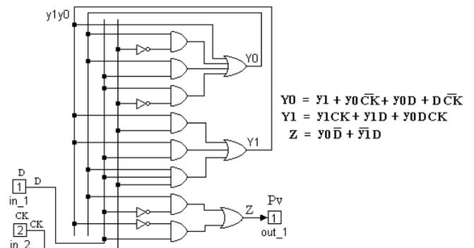
Figure 3. Intern aspect of the block  $P_v$
