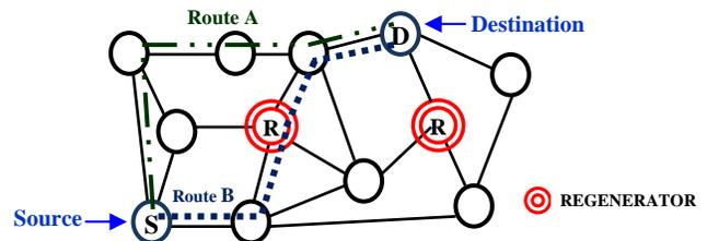
Figure 1. Example of routing in a translucent optical network.
