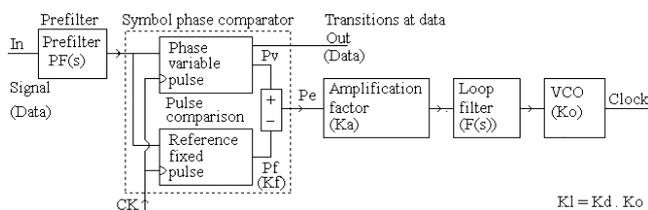
Figure 1. Prefilter with synchronizer based on pulse comparison
