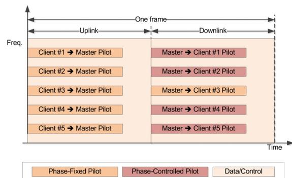
Fig. 2. Frame Structure
