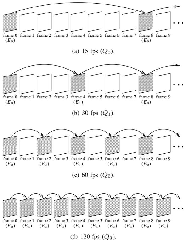
Figure 1. Hierarchical decoding of one-dimensional scalable medium X at frame rate  $Q_{d_1}$  ( $J = 1$  and  $D_1 = 4$  ( $d_1 = 0, 1, 2, 3$ )).
