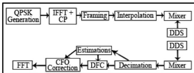
Figure 1. Baseband and IF transceiver architecture
