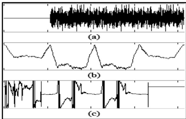
Figure 4. Estimation algorithm results for a frame with 3 OFDM symbols: (a) signal, (b) peak detection and (c) computed angle.
