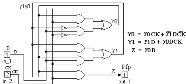
Figure 10. Intern aspect of the block Pfp
