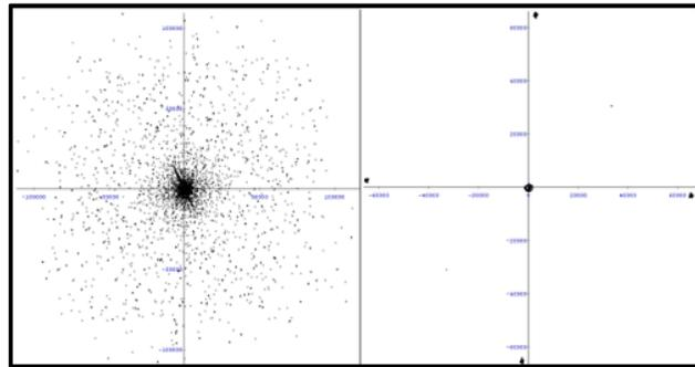
Figure 5. OFDM symbol with a 6 kHz offset between oscillators. Before compensation (left) and after compensation (right).
