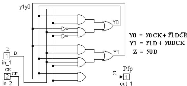
Figure 12. Intern aspect of the block Pfp
