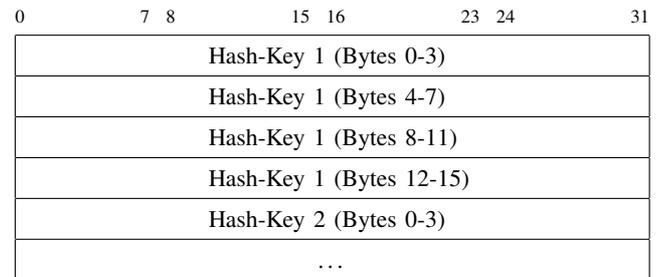
Fig. 9. Body structure of COLERR messages
