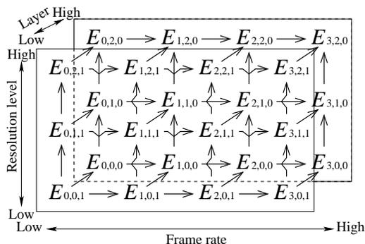
Figure 6. Decoding order of entity  $E_{d_1, d_2, d_3}$  in three-dimensional scalable medium  $X$  ( $J = 3$ ,  $D_1 = 4$ ,  $D_2 = 3$ , and  $D_3 = 2$ ).
