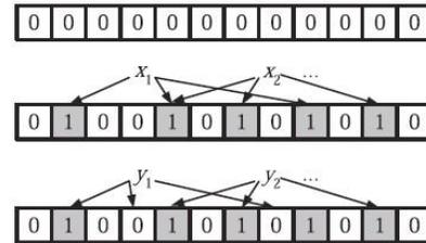
Figure 2. An example of a bloom filter taken from [8]. The filter begins as an array of all 0s. Each item in the set  $x_i$  is hashed  $k=3$  times, with each hash yielding a bit location; these bits are set to 1. The element  $y_1$  is not in the set, since a 0 is found at one of the bits. The element  $y_2$  is either in the set or the filter has yielded a false positive.
