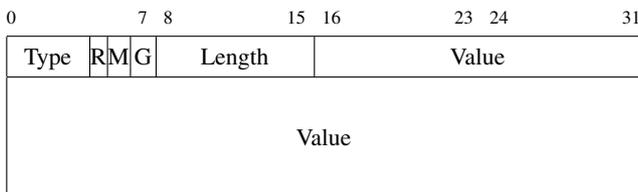
Fig. 8. Body structure of NADV messages
