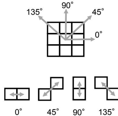
Figure 2. Extraction of Multi-direction pixel pairs .
