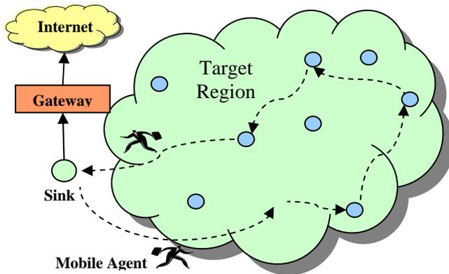
Figure 2. Mobile agent-based wireless sensor network
