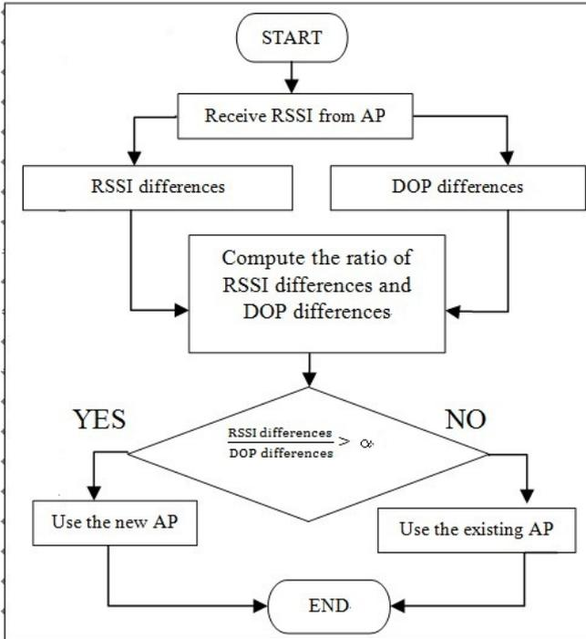
Figure 4. The proposed positioning algorithm.
