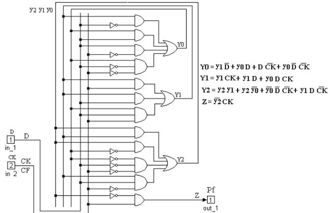
Figure 6. Intern aspect of the block Pf
