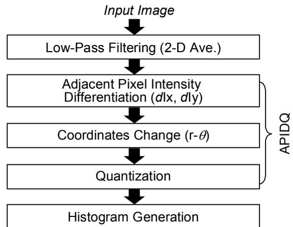
Figure 1. Processing steps of APIDQ histogram method.
