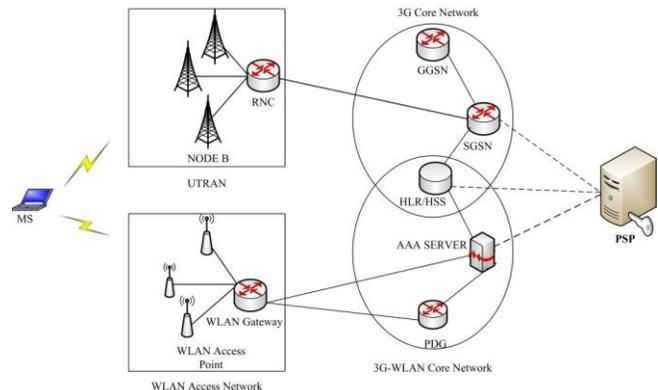
Figure 1. PRIPAY deployment in a 3G-WLAN integrated network
