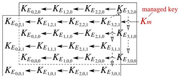
Figure 7. Key assignment to control access to three-dimensional scalable medium  $X$  shown in Fig. 6. Solid arrows are OHCs and dashed arrows represent MHCs.
