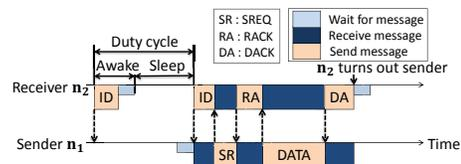
Figure 3. Procedure for forwarding data in IRDT
