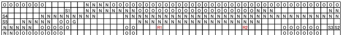
1cell = 10m × 10m, N: the relays installation impossible, O: the obstacles, S: the wireless sensors' location
