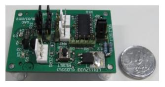
Figure 4. Intelligent Sensor Module (ISM).
