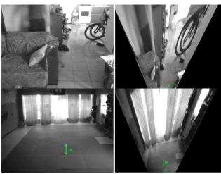
Figure 4: Input images and their inverse perspective transformation mappings
