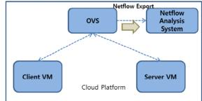
Figure 1. Cloud-based Netflow Collection System.
