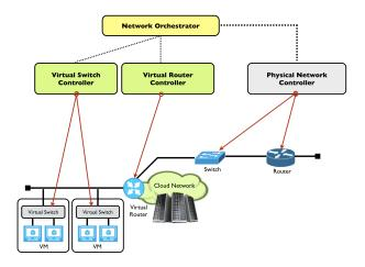
Figure 3. Network control architecture for E2E service chaining
