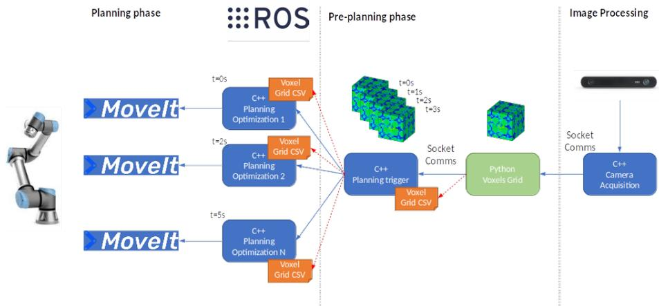
Fig. 3. Path planning solution architecture and module relationship.
