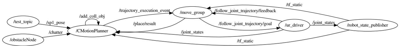
Fig. 6. rqt\_graph view of the nodes and topics involved in actuating the model.
