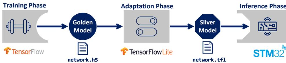
Figure 1. General and exemplary interaction between Training Phase, Adaptation Phase, Inference Phase, Golden Model and Silver Model.
