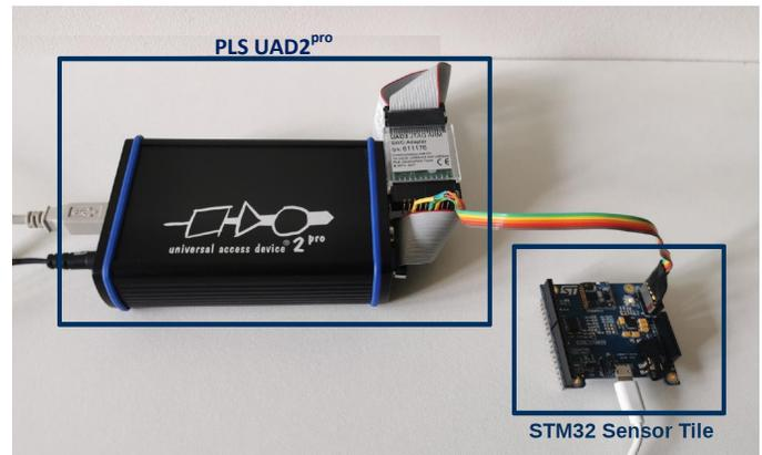
Figure 3. STM32 Sensor Tile connected to the PLS UAD2<sup>pro</sup>.
