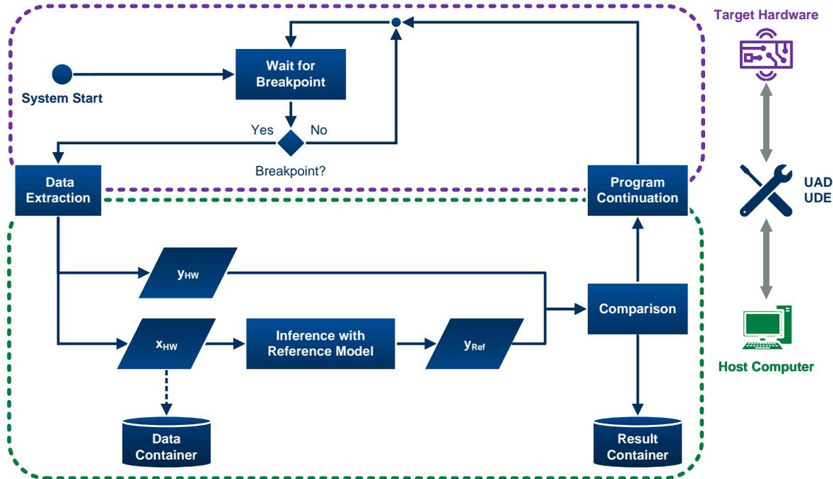
Figure 2. Schematic structure of the diagnostic loop for the continuous comparator-based analysis of the hardware and model outputs. Purple dashed frame: Processes belonging to the context of the target hardware. Green dashed frame: Processes belonging to the context of the host computer.
