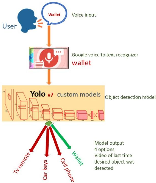
Fig. 2. High-level architectural view of the approach.
