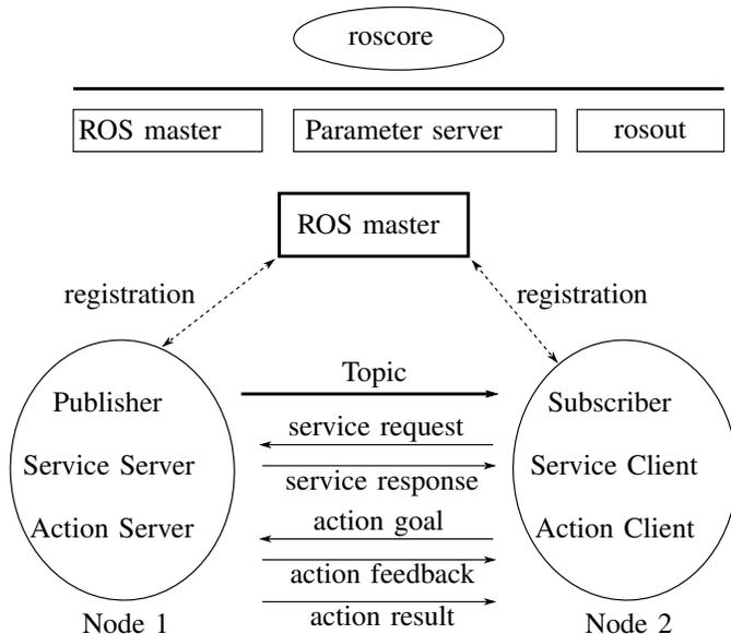
Fig. 2. ROS core communication system, and different message communication modes between nodes (adapted from [17]).
