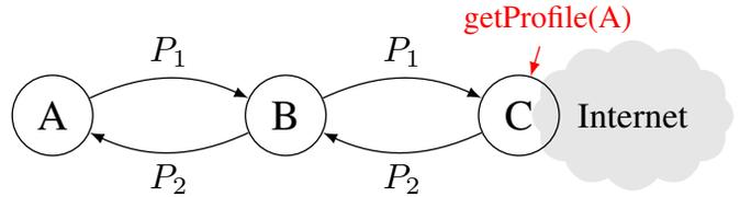
Figure 4. Applying utility function at replying node. **A** – CARMNET node, **B** – CARMNET Relaying node, **C** – CARMNET Internet Sharing node,  $P_1$  – Virtual price calculated at Node A,  $P_2$  – Virtual price calculated at Node C
