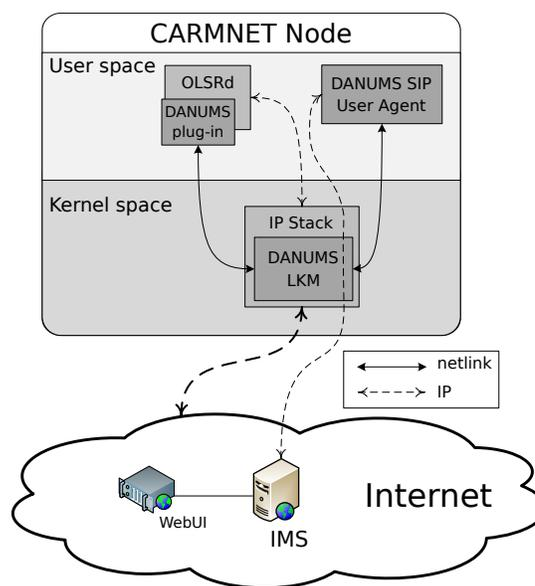
Figure 1. Architecture of the CARMNET network [3].
