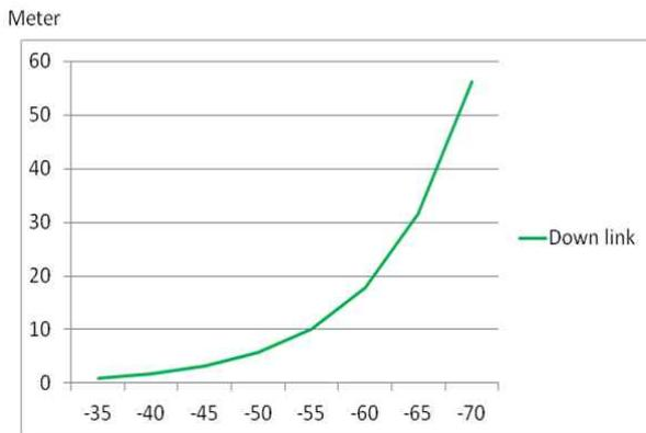
Figure 3. Signal transmission coverage for various RSSI values
