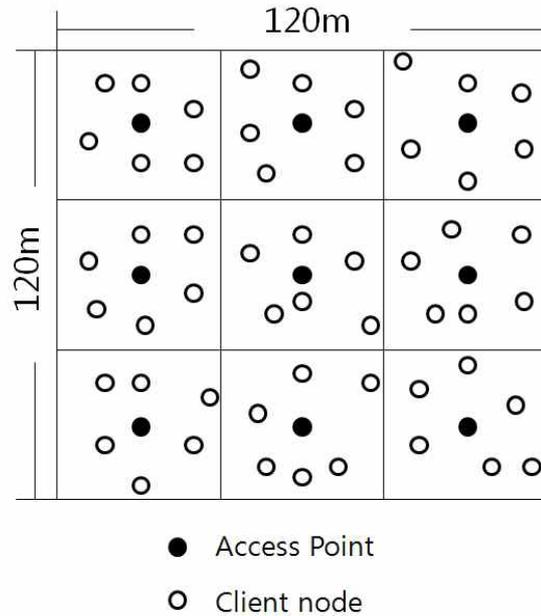
Figure 6. Simulation topology with 9 cells and 54 devices
