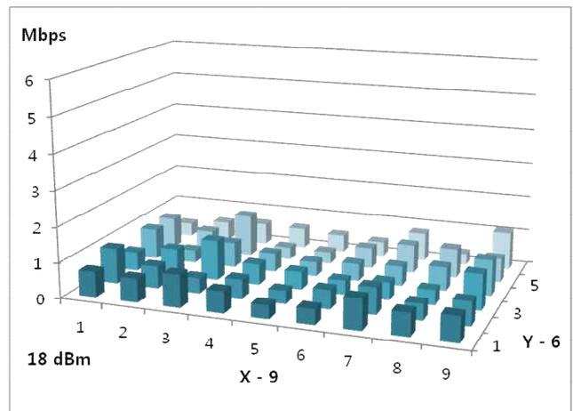
Figure 7. Throughputs at randomly located 54 clients with 18dBm transmission power
