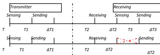
Figure 2. The RTS based channel reservation scheme.
