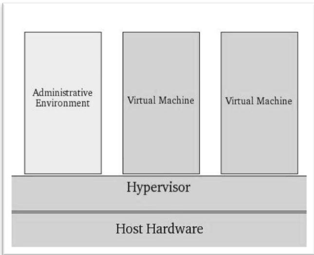
Figure 2. Virtualization Hypervisor Layer (Source: Virtuatoopia, 2009)
