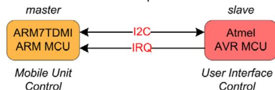
Figure 5. I2C communication protocol block diagram
