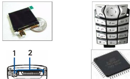
Figure 2. User interface parts a) LCD b) matrix keyboard c) output connector d) MCU and Flash
