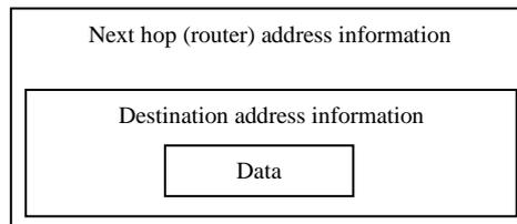
Figure 1. Model of a frame and some conceptual layers in computer networking
