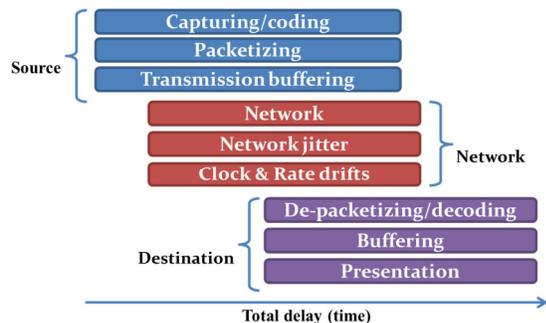
Figure 1. End-to-end causes of delay.
