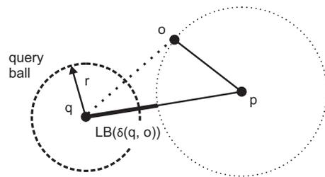
Fig. 2. Lower-bound estimation using a reference point  $p$ .
