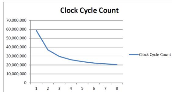
Figure 7. Performance Test (clock cycles / no of cores).
