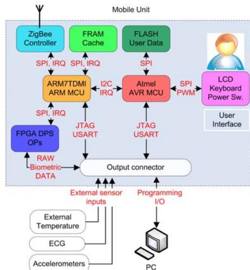
Figure 1. The mobile unit block diagram
