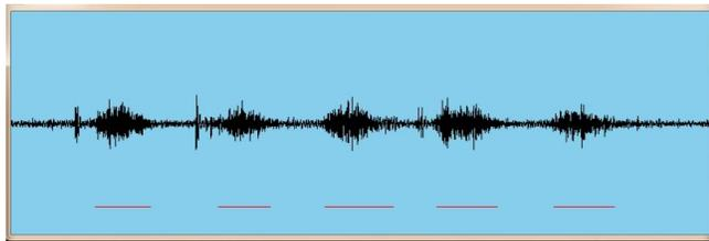
Figure 2. A vibration wave signal recorded by our experiment system where straight line segments denote the corresponding time when soft whisper is being pronounced.
