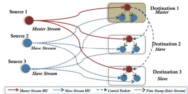
Figure 4. Master/Slave Receiver Scheme (MSRS).
