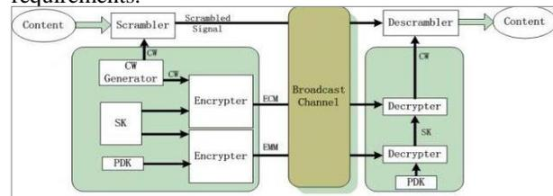
Figure 1. typical Conditional Access System [14].
