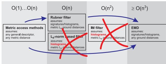
Fig. 3. Filter chain used in the filter-and-refinement scheme for EMD search.
