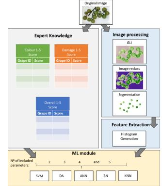
Figure 2. Summary of image processing and ML tools for the multimedia monitoring system for grape quality detection.
