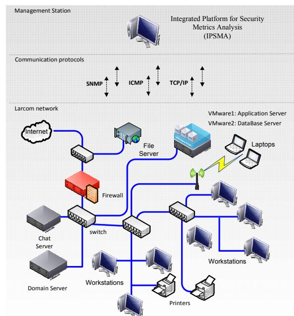
Figure 6. Real network following the proposed architecture
