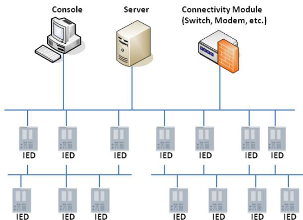
Figure 2. Bus Topology in an Industrial Network
