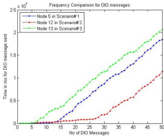
Figure 4. Frequency Comparison of DIO messages sent by Malicious nodes and Counterparts
