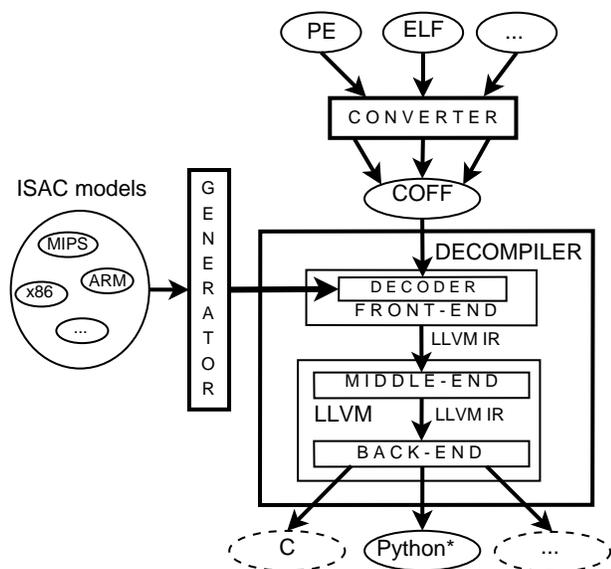
Figure 1. The concept of the Lissom project's retargetable decompiler.
