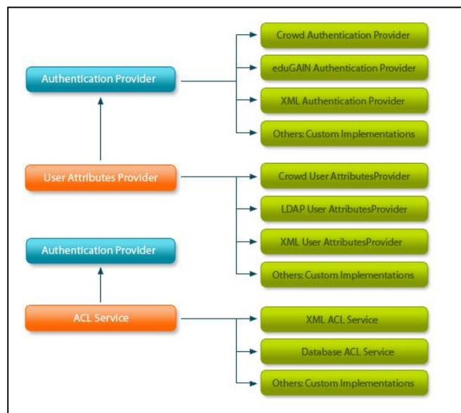
Figure 2. The architecture of AA Framework [20]
