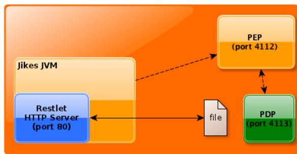
Figure 3. BonFIRE Compute Resource with integrated PEP module
