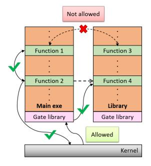
Figure 1. Memory segmentation and access control
