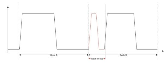
Fig. 1: Injection of a Clock Glitch
