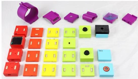
Figure 4 Packages for attachable and wearable applications.
