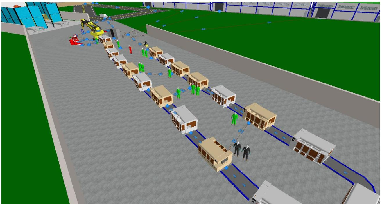
Figure 2. Model Animation Showing the Revised “U”-Shape of the Assembly Line
