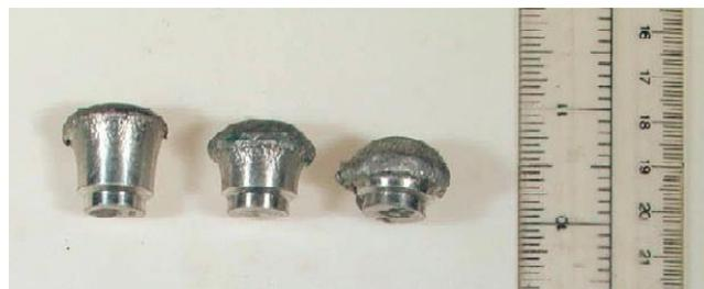
Figure 7. Deformed 6061-T6 aluminum projectiles after perforation 0.125, 0.25, and 0.5 inch thick (left-to- right) aluminum targets.
