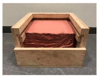
Figure 4. Shooting-box filled with plasticine. Inner dimensions: 250 mm x 300 mm x 15 mm.
