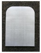
Figure 2. Side body pattern out of Dyneema® HB26. Width of 150 mm and a total height of 205 mm.
