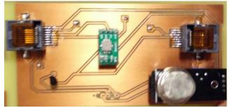
Figure 5. Sensor printed circuit board
