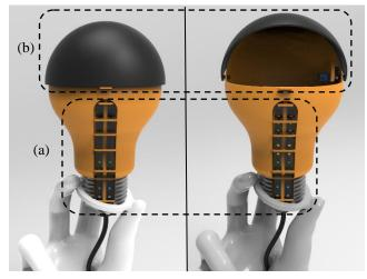
Figure 4. Opening mechanism (b) and lighting of leds (a)
