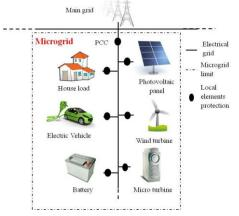
Figure 1. Example of Microgrid structure
