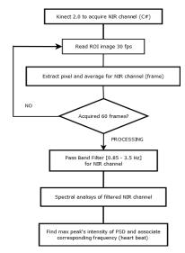
Figure. 1. Block diagram real-time processing NIR channel.
