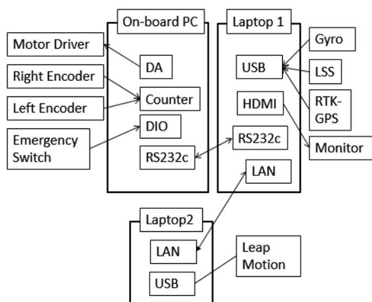
Figure 3 System Configuration
