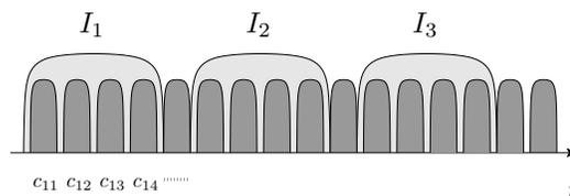
Fig. 4. Interference Scenario. Each interfering carrier  $I_i$  induces a certain packet error probability over the overlapping IEEE 802.15.4 channels.
