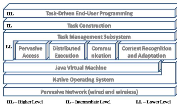
Figure 2. System architecture for tasks managing and programming
