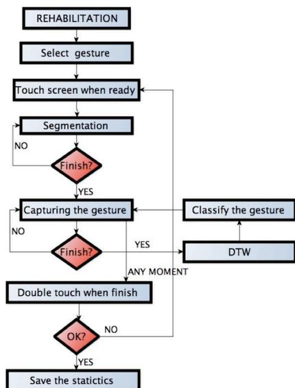
Figure 4. Flow chart that represents the steps to perform the rehabilitation process.
