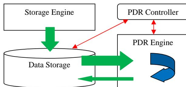
Figure 1. Interaction of main PDR components [2]
