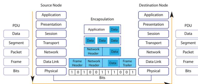
Figure 1. Encapsulation process in communication between nodes
