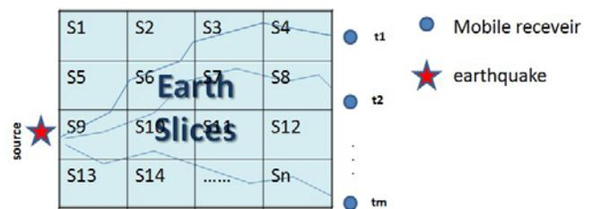
Figure 1. The discrete slowness model for seismic tomography.
