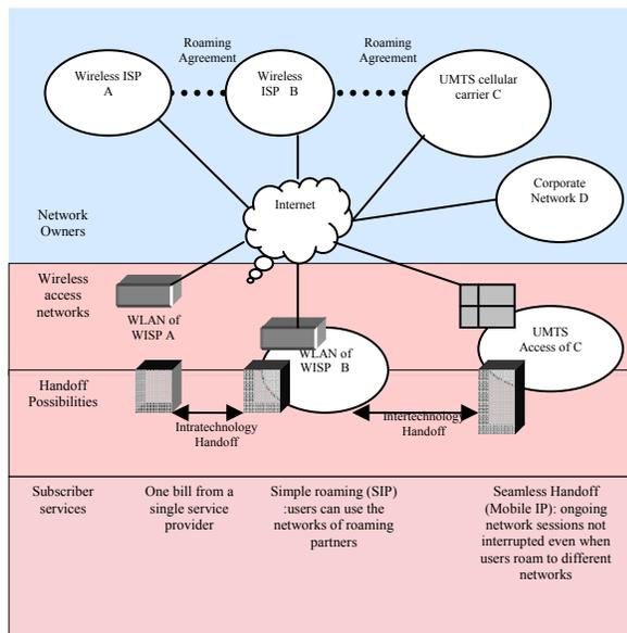
Figure 6: WLAN-UMTS Interworking (adapted from [12])
