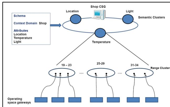
Figure 2. Illustration of the Overlay Structure.
