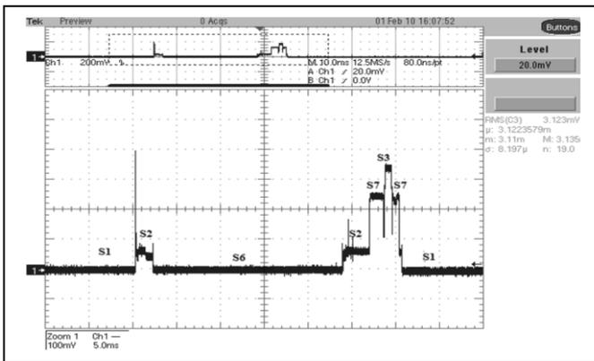
Figure 5. Oscilloscope output for a noise-free channel
