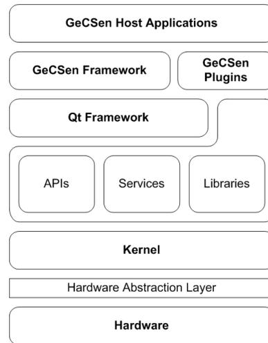
Figure 2. GeCSen on top of OS Architecture
