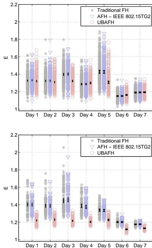
Fig. 9. Energy performance for traditional FH, IEEE AFH and UBAFH in a real environment. Results have been obtained considering 100 (top) and 500 (bottom) packet transmissions. 95% confidence intervals are also shown. Note that day 6 and 7 correspond to Saturday and Sunday
