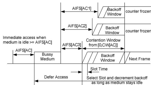
Figure 2. IEEE 802.11e EDCA mechanism [6].
