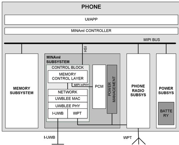
Figure 3. MINAmI Architecture on phone
