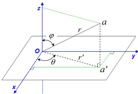
Figure 3. Spherical coordinates
