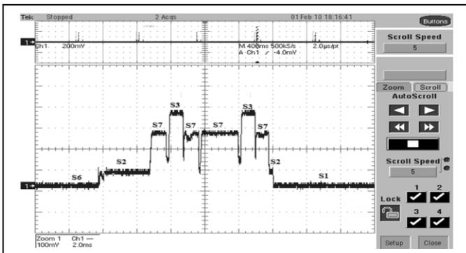
Figure 6. Oscilloscope output for a noisy channel due to a noisy channel the first transmission was unsuccessful and following retransmissions were required. The states S1 to
