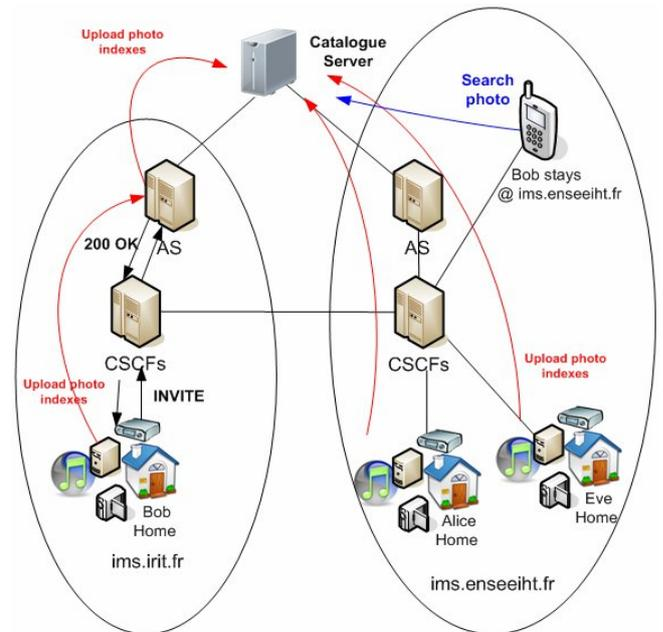
Figure 2 : Photo sharing with IMS Architecture
