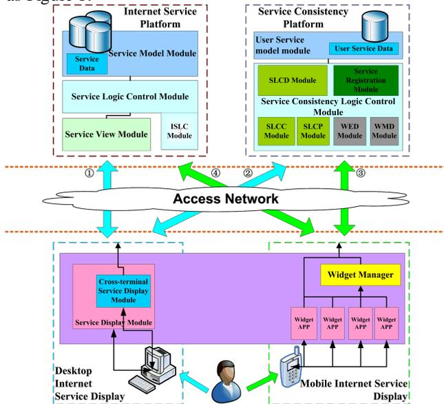
Figure 1. The components of service consistency framework
