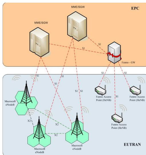
Figure 4. E-UTRAN Architecture including the deployment of Femtocell
