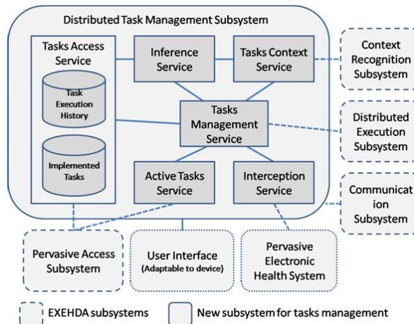
Figure 3. Architecture of the Tasks Distributed Management Sub-system
