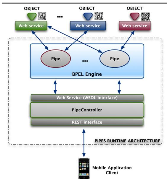
Figure 4. Hyperpipes at runtime. Objects are instrumented by Web services and Pipes are implemented as WS-BPEL processes created and deployed at runtime. A mobile phone is used to point objects in the environment and to retrieve the WSDL specification.
