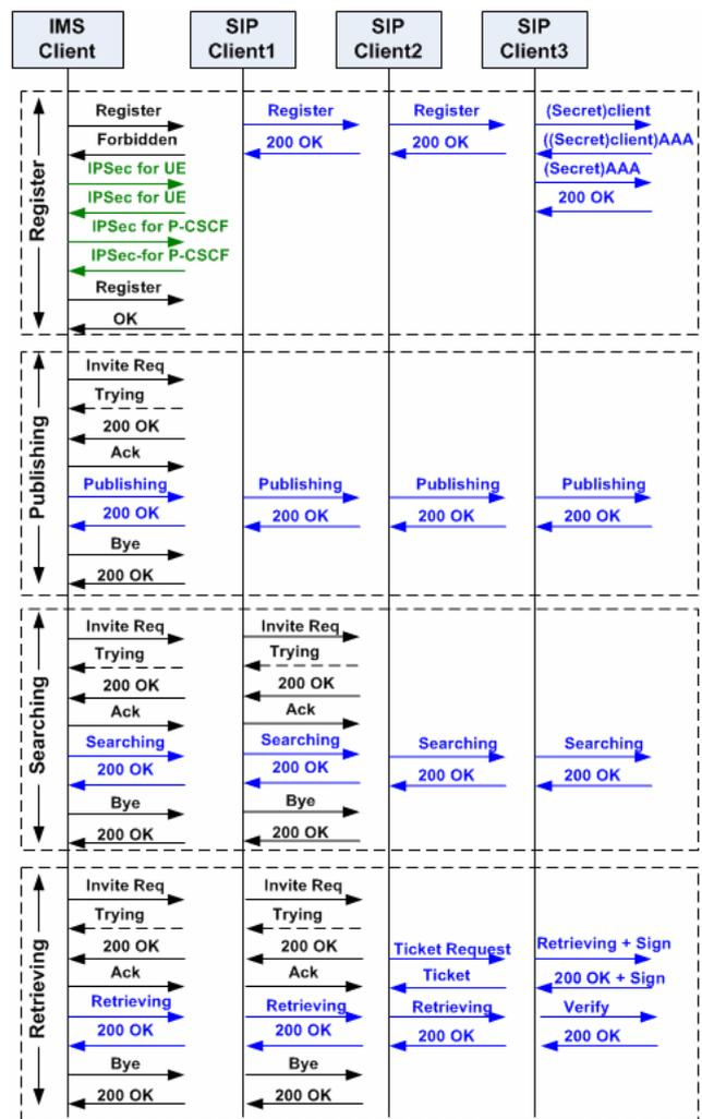
Figure 6: Client signalling
