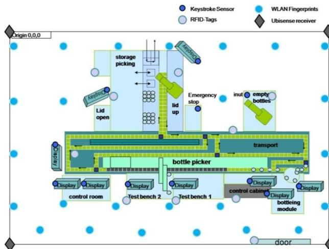
Figure 4. Schematic overhead shot map of the SmA with integrated sensor sources for location determination
