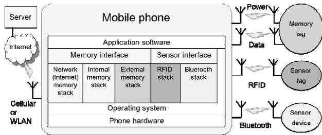
Figure 1. MINAmI Architecture
