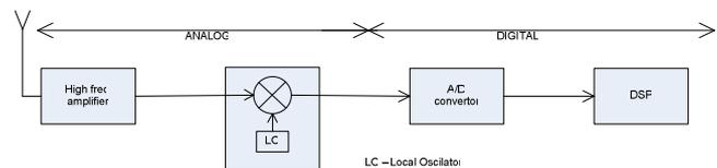
Figure 2. Block diagram of Software Defined Radio
