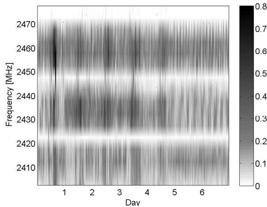
Fig. 2. Average channel occupancy for the 16 IEEE 802.15.4 channels during a 7-day period, from April 19 to April 25.
