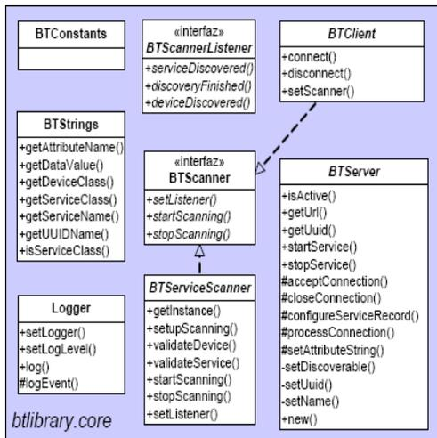
Figure 2. Classes and components of btlibrary.core
