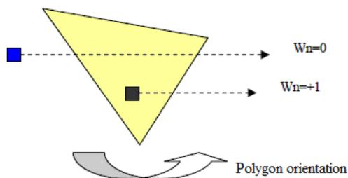
Figure 3. The application of Winding number method
