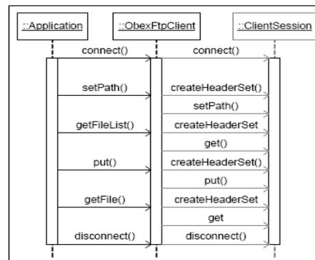
Figure 4. Message sequences in a OBEX FTP service.
