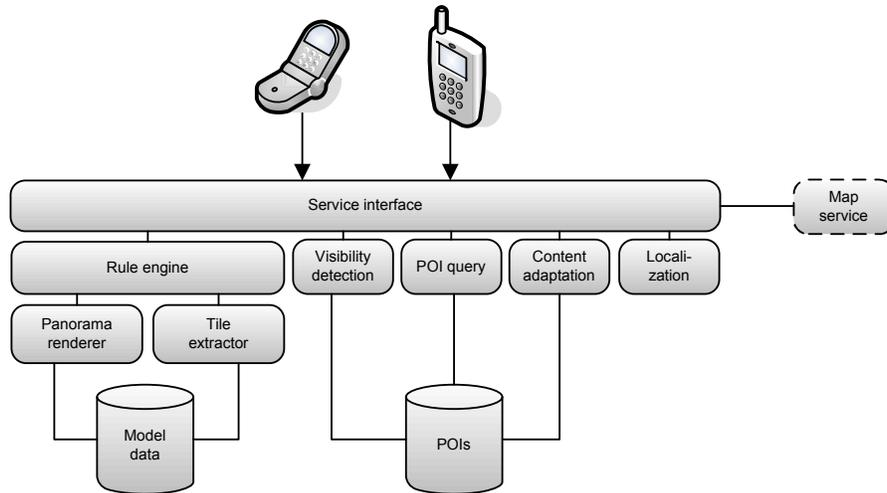
Fig. 1. Components of the proposed device-aware visualization platform.
