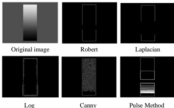
Figure 3. Results of edge detection methods compared to the result of pulse domain technique (right-bottom one).
