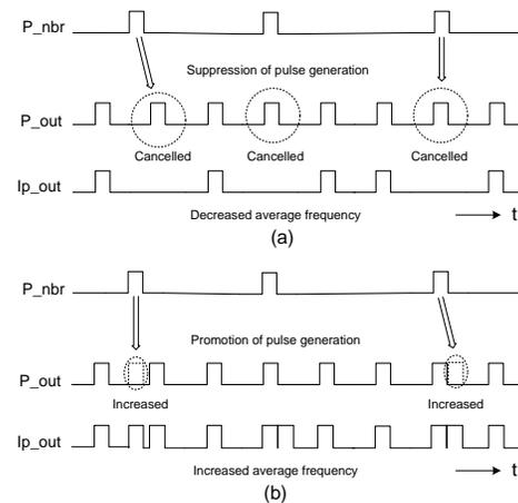
Figure 2. Processing operations in pulse domain: (a) suppression and, (b) promotion algorithms.
