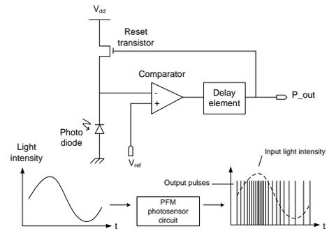
Figure 1. Architecture of PFM photosensor
