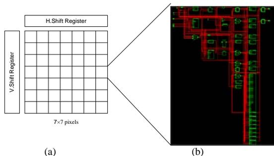
Figure 9. (a) Schematic diagram of an array, (b) RTL schematic per pixel
