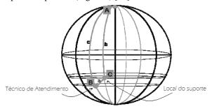
Figure 1. Arcs to calculate the length between two points using spherical trigonometry.
