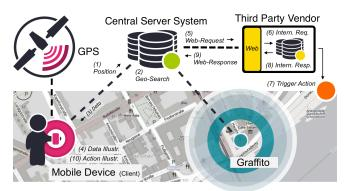
Figure 1. System Architecture for Proximity-Triggered Code Execution
