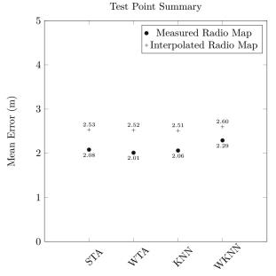
Figure 7. Mean Positioning Error of all Algorithms of Test Scenario II
