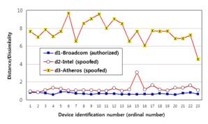
Figure 4. Performance of MAC spoofing attack detection against mobile devices with different Wi-Fi chipset.
