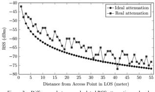
Figure 3. Differences between calculated RSS attenuation and real recorded attenuation
