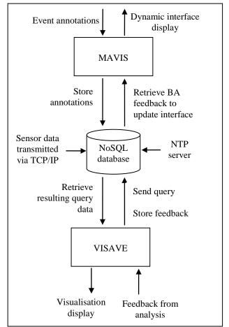
Figure 1 - A sequence diagram showing how data flows through the system.
