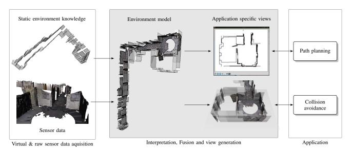
Fig. 3: Composing an environment representation from static & dynamic data and generate of application specific views from it.
