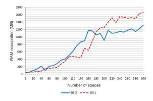
Fig. 10: SIS 2 vs SIS 1: memory footprint comparison
