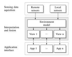
Fig. 2: View generation related to application requirements and based on a common environment representation.
