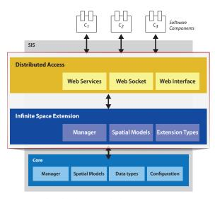
Fig. 5: The extended SIS Structure
