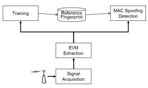
Figure 2. Architecture for MAC spoofing attack detection.
