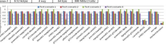
Figure 2. EDP normalized to the homogeneous core system (baseline of one) for the test scenarios in Table 2
