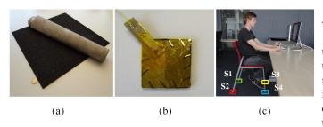
Fig. 1. System Design; a) raw materials for the pressure sensor; b) a sensor prototype; c) a chair equipped with sensors
