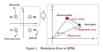
Fig. 1 shows digital modulation error in QPSK. QPSK can send two bits of digital information at a time. In QPSK, data is encoded using two independent carrier components, in-phase (I) and quadrature phase (Q). The carrier
