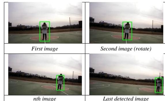
Figure 12. Examples of Image Sequence and pedestrian detection (5.5m, stationary pedestrian)
