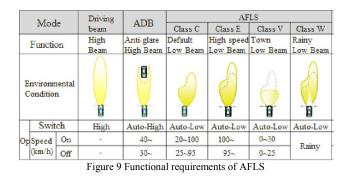
The ECU of intelligent headlamp system receives environmental information, such as vehicle speed, illumination and other vehicle, from other ECUs and controls the headlamps of vehicle. At the first phase, the functional requirements are elicited from informal documents that contain functional and non-functional requirements for ECU, R.48 and R.123 of UNECE, and described in MS word. The
