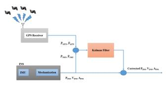
Figure 1. INS/GPS Integration in Loosely Coupled scheme
