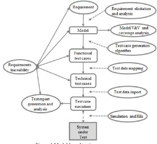
Figure 1 Model-based testing process
