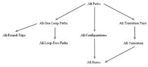
Figure 2 Transition based test coverage
