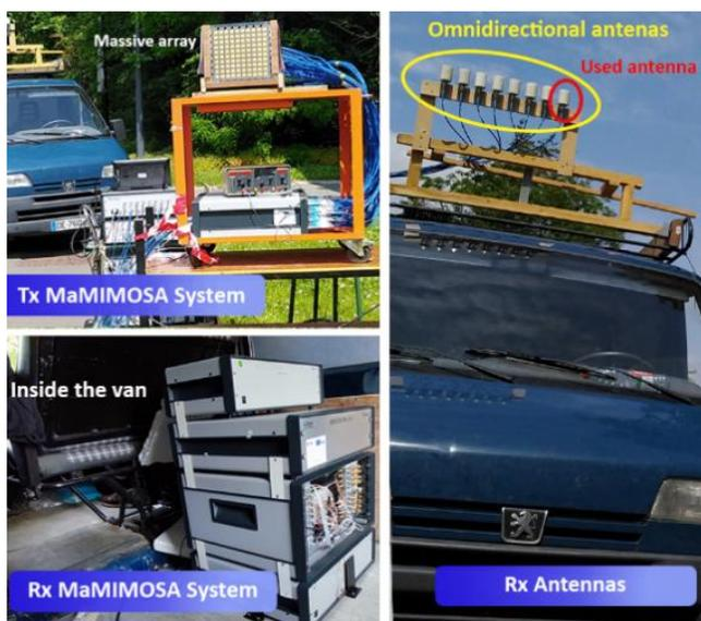
Figure 2. Tx-Rx antenna systems.
