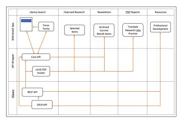
Figure 1. REACH System Architecture.
