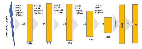
Figure 3. CNN Pitch Detection.
