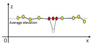
(b) Fixing elevation anomalies. Nodes in isolated groups are adjusted to the average elevation level.
