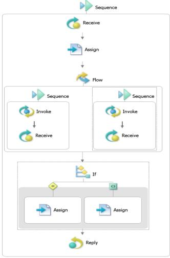
Figure 1: BPEL View of Loan Application Process
