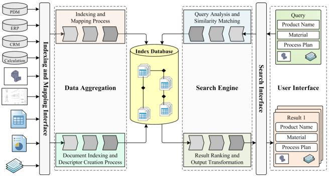
Figure 2. Architecture of integrated content-based enterprise search (CBES)
