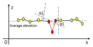
(a) Identifying elevation anomalies. Two isolated groups (in red) and angles ( $\alpha$ 1 and  $\alpha$ 2) resulting from the difference between the area-weighted normal vectors
