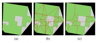
*Figure 5:* Illustration of the topological abstraction process with a strict convex property (C(gr) = 1); (a) the GIS data of a complex building; (b) the exact space decomposition using CDT techniques (63 triangular cells); (c) the topological abstraction (28 convex polygons)
