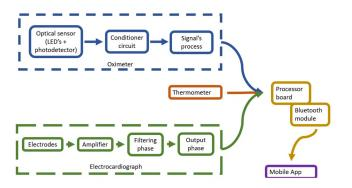
Figure 1 Delphi's block diagram.
