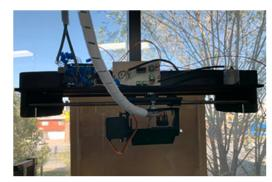
Figure 5. Final protype of the temperature acquisition system.
