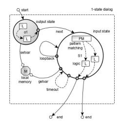
Figure 2. Naifjs dialog manager. Dialog with a single input state (on the left). 2-states dialog (on the right).
