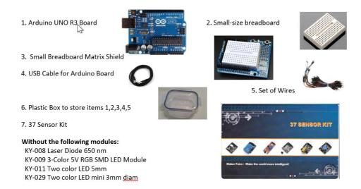
Figure 1. A list of electronic components that were provided to the students for the work at their homes.
