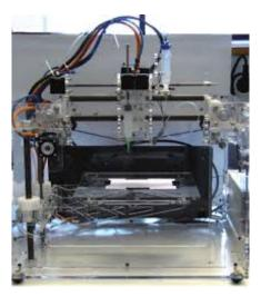
Fig. 5: Open-source design 3D printer
