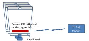
Figure 2. Scheme for detecting an empty bag using RFID
