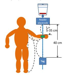
Figure 9. Image of electric-field between reader electrode, tag and earth via human
