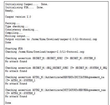
Fig. 2. Verification result of the LA protocol using Casper/FDR2
