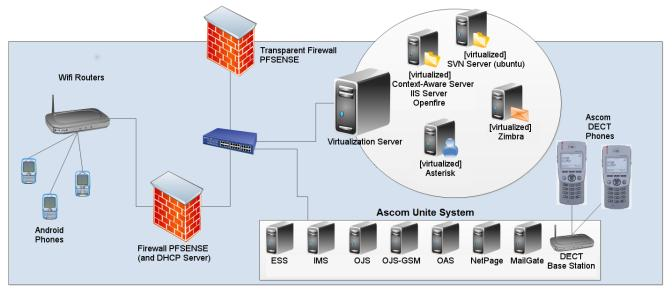
Figure 2: CallMeSmart prototype network structure
