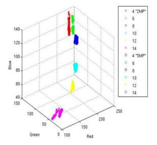
Figure 3. Distance between the camera and the HCS is approximately 7.5 cm (camera screen spans the preview of the HCS). Camera's MP settings are 2 MP and 5 MP.
