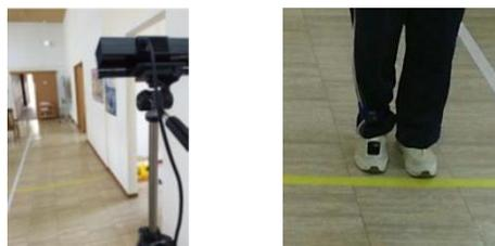
(a) MS-KINECT set up in rehabilitation facility (b) WD mounted on stroke patient
