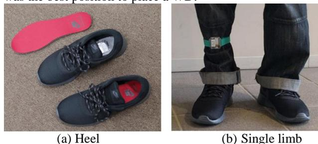
Figure 8. WD attaching position
